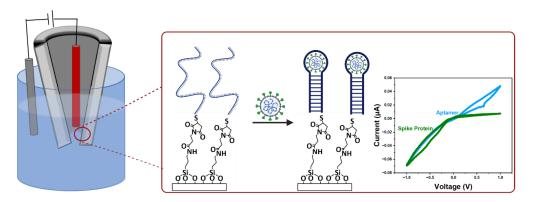
**Figure 1:** Schematic of an aptamer functionalised nanopipette surface, and a representative voltammogram of the successful detection exploiting an aptamer conformational change and the surface charge dependence of ICR.
