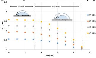
Fig. 1 Experimental results of the frequency shift ( $\delta f$ ) of ultrasonic sensor, covered by Ti film, during evaporation of a 2  $\mu$ L water droplet, measured in various frequencies as a function of time at room temperature. Two modes of evaporation (pinned and unpinned) can be well distinguished.
