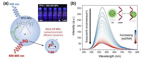
Figure 1 (a) Schematic representation of the composite particle system and studied dynamics and image of NP suspensions with 0-5 wt% SQ dopant under UV irradiation showing gradual colour change due to ET. (b) increasing luminescence quenching with addition of ssDNA showing schematic interaction between DNA and oPD CDs.
