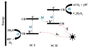
Fig. 1: schematic representation of the AP reaction mechanism using z-scheme photocatalysis where a) is photon absorption, b) is neutralisation and charge carrier separation, c) is H<sub>2</sub>O oxidation, d) is CO<sub>2</sub> reduction.
