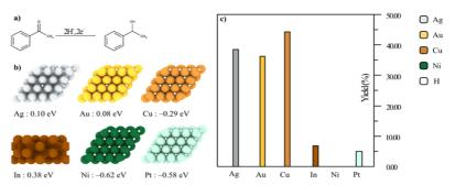
Figure. a) ECH of AC to 1-phenylethanol. b) Top views of the H surface coverages predicted under ECH conditions. c) Experimental ECH yields
