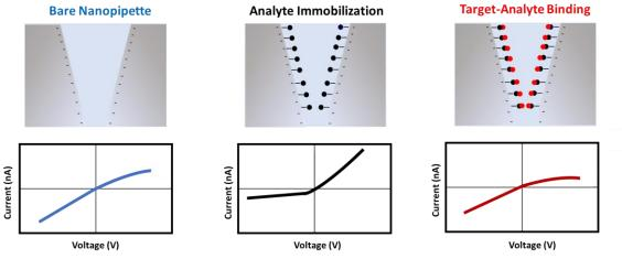
*Figure 1.* A representation of the sensing approach based on exploiting the surface charge dependence of ICR.
